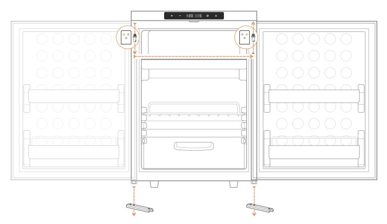
Unscrew the lower door hinge and the base on the opposite side. Then pull the appliance door downwards.
