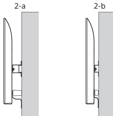
3 Refer to the below table about the Base Adaptor fitting location. In case of selecting 2-b, then skip this step.
