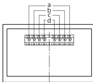
Fit Base Adaptor ① by using Screw (PSW 4x10) ② to Base (20) ③ when selecting 2-a.
