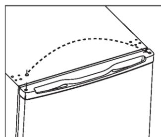
6. Remove the screws and bottom hinge. Then remove the adjustable feet from both side.
