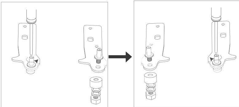
8. Refit the bracket fitting the bottom hinge pin. Replace both adjustable feet.
