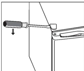
5. Move the core cover from left side to right side. And then lift the door and place it on a padded surface to prevent it from scratching.
