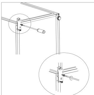
9. Place the door back on. Ensure the door is aligned horizontally and vertically so that the seals are closed on all sides before finally tightening the top hinge.
